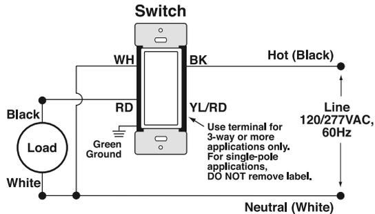
**THREE-WAY WIRING DIAGRAM**
