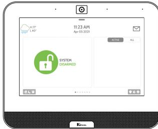
To access the Advanced Settings menu pull down the Settings tray at the top of the screen, select “Settings” and then “Advanced Settings”. Enter your dealer, installer or master code. The code used to enter Advanced Settings determines the level of access. When using partitions the code entered at the screen lock determines the access level for Advanced Settings.
