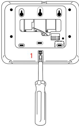
1. With a small Phillips screwdriver, undo the locking screw from the back of the panel, remove the SmartMount backplate and discard.
