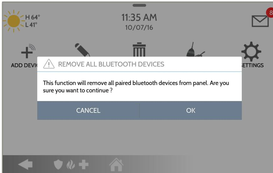
To delete and remove all enrolled Bluetooth devices at once, select “Remove All Devices”.
