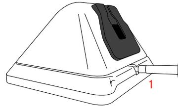
1. With a small Phillips screwdriver, screw in the locking screw from the bottom of the panel to secure it to the IQ Base.
