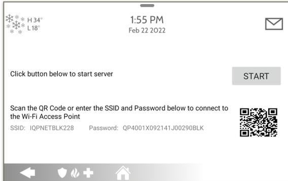
1- Scan the QR Code with your phone camera or manually connect to the Panel AP with the SSID and Password shown on the screen.
