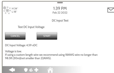
If voltage is below 6vDC, you will receive a “Voltage is Low” message and action should be taken to correct the low voltage condition (i.e. use thicker gauge wire or shorten the wire run).
