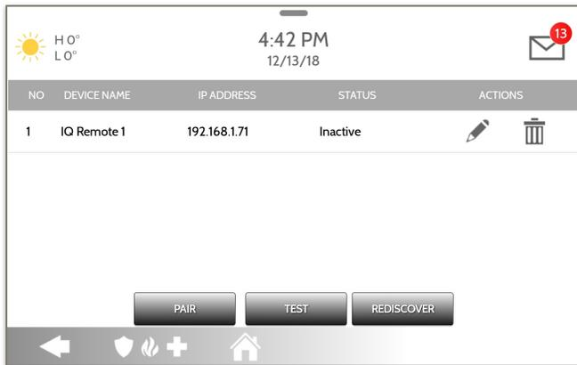
**NOTE:** The IQ Remote will automatically pair as Sensor Type “Keypad” and will appear on the zone list in the order in which it is paired. Sensor Groups 0, 1 & 2 are available options for this Sensor Type.
