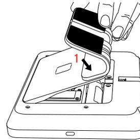
1. Locate the SmartMount table stand and insert the hooks into the back of the panel, then swing down and press into place.
