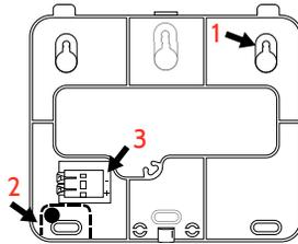
1. Mount the backplate to the wall using flat head screws\* and appropriate wall anchors if needed, ensuring it is level.
