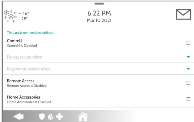
Check the “Control4” box to enable 3rd Party Connections. This will cause the panel to reboot in order to apply the change. Once enabled a secure token can be generated in order to sync with Control4 integration.
