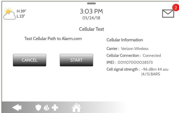
To begin the test press "Start" and watch for the results on the screen.
