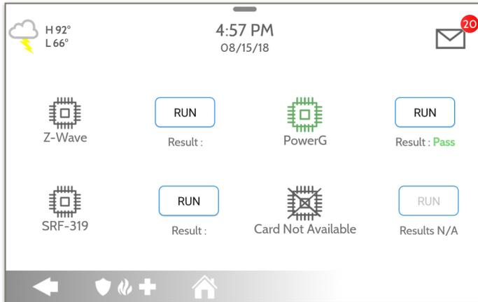
Select “Run” on an individual available card to start the test. In some cases the test may take several minutes after which the panel will show a result of a “Pass” or “Fail”.
