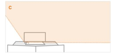
3. Thread the existing wires through the mounting bracket. Install the mounting bracket to the wall using the included wall screws (and anchors, if needed for the mounting surface).
