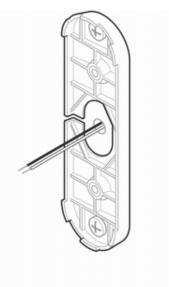
6. Install the doorbell backplate to the mounting bracket using the included machine screws.
