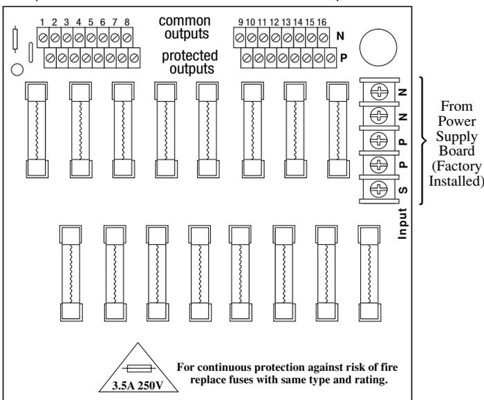
*Fig. 4b - PD16WCB - Power Distribution Board
