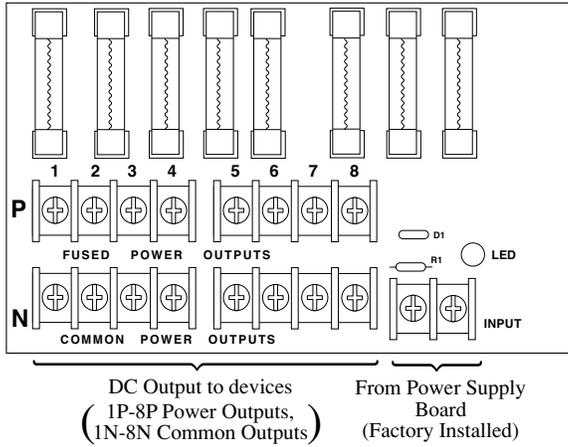
*Fig. 3b - PD8ULCB - Power Distribution Board
