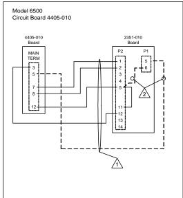
4 conductor, stranded with overall shield, 18, 20, 22 or 24 gauge is sufficient for these connections.
