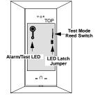
powering the unit off and then on or by placing a magnet over the reed switch (can be done with cover in place). Placing a magnet over the reed switch when the unit is in the test mode will terminate the test.
