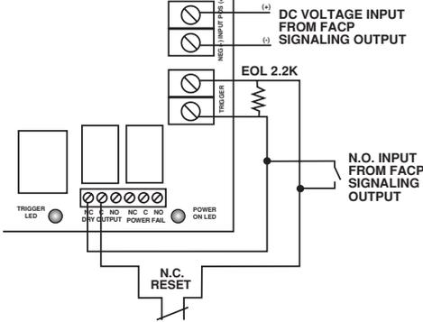
MOM5 module shown with with wet and/or dry normally closed fire alarm trigger inputs
