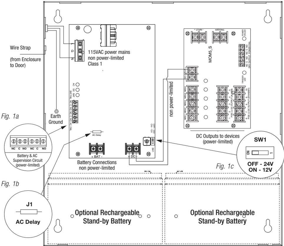
Keep power-limited wiring separate from non power-limited. Use minimum 0.25" spacing.
