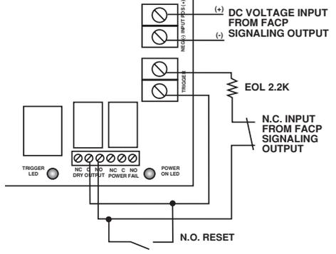
Fig. 9 - Two (2) MOM5 modules shown with wet and/or dry normally closed fire alarm trigger inputs
