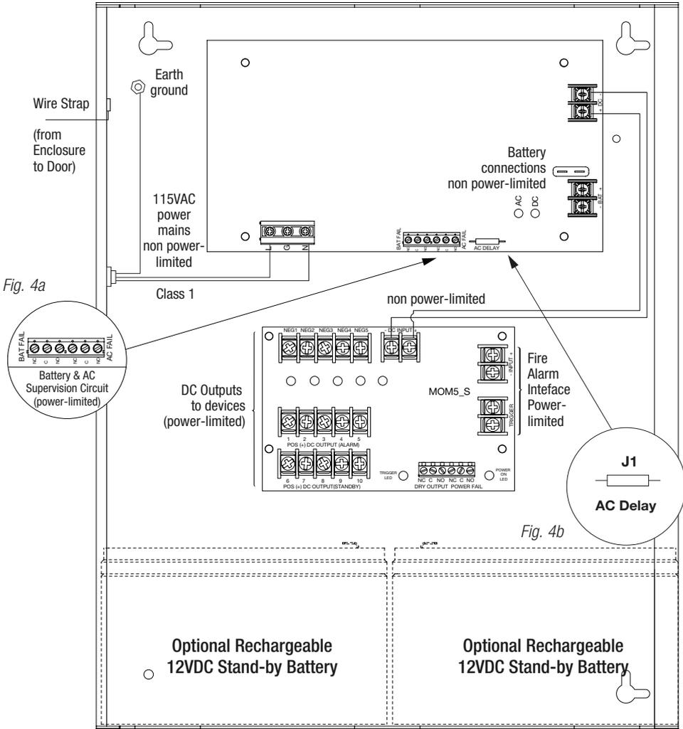
Keep power-limited wiring separate from non power-limited. Use minimum 0.25" spacing.
