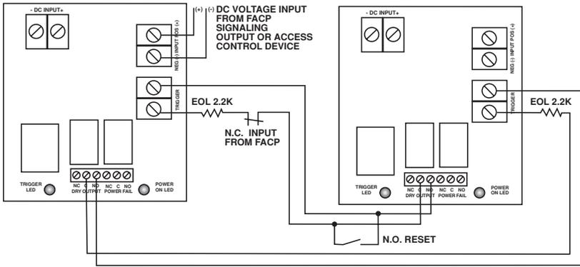
Fig. 10 - Two (2) MOM5 modules shown with wet and/or dry normally open fire alarm trigger inputs
