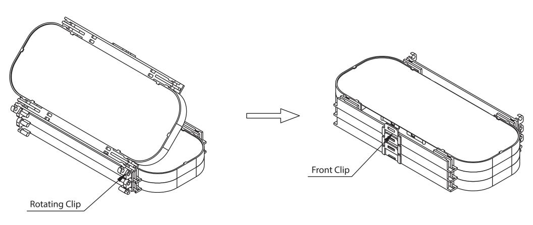
When installing or removing the splice trays, release the front clip allowing the top splice tray to be angled at a 45° so that the rotating clip on the back of the splice tray can be unsnapped from the lower plate.
