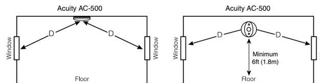
**NOTE:** Maximum distance 'D' is limited by the range (refer to the Glassbreak Detector Range chart)
