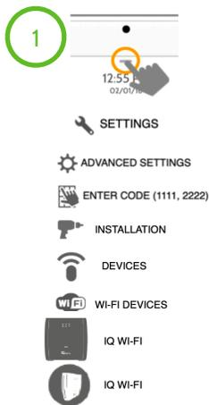
Open settings tray, touch settings, advanced settings, type valid code, touch installation, devices, WI-FI devices, IQ WI-FI, IQ WI-FI
