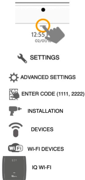
Open settings tray, touch settings, advanced settings, type valid code, touch installation, devices, WI-FI devices, IQ WI-FI
