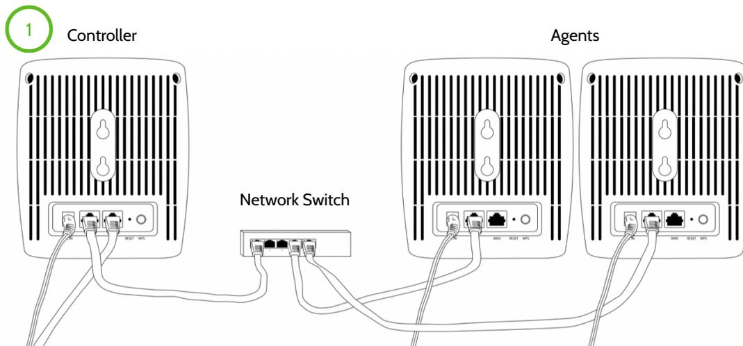
1. Add a network switch (not provided) to add multiple Agents to a Controller for configuration. Once powered and physically connected with the provided ethernet cable the connected Agents will auto configure and update based on Controller device settings. Adding a switch will help speed up larger router installations.
