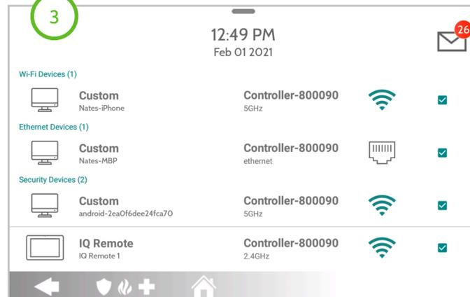
*\*Note: When viewing connected devices, you can manage internet connectivity by unchecking (not internet) the checkbox of a connected device.*
