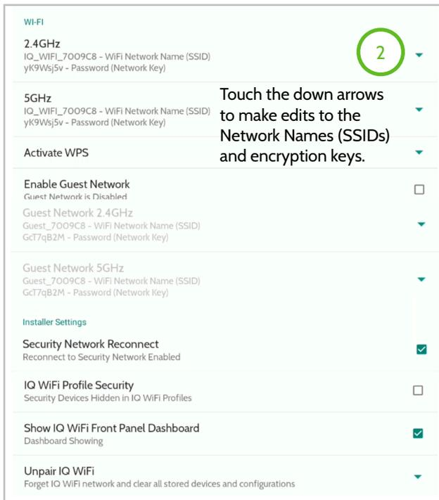
Touch the down arrows to make edits to the Network Names (SSIDs) and encryption keys.
