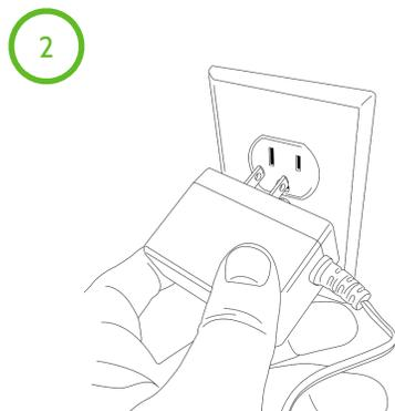
Plug the barrel jack end of the power supply into the DC-IN and plug the power supply into the wall outlet. Router takes 6 minutes to power up, the Power LED will stop flashing when ready.
