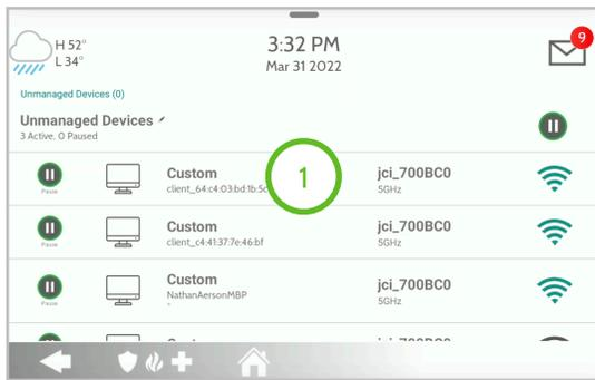
1. To change the profile for each device touch the device name.
