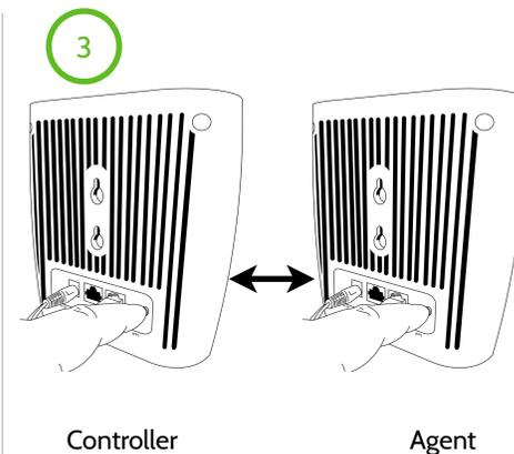
Once the Agent is powered the LEDs are solid GREEN. Activate WPS on the controller by pressing and holding the WPS button for about 1 second then press the WPS button on the Agent for about 1 second. The pairing process can take up to 7 minutes to finish pairing. You can begin pairing subsequent Agents when the Controller WAN LED goes solid GREEN.
