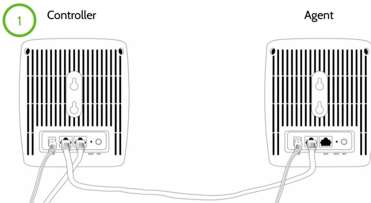
1. With a Controller already powered and connected, add an Agent to a Controller by using the provided ethernet cable. Plug each end of the ethernet cable into the LAN port of both the Controller and the Agent creating a LAN-to-LAN connection.
