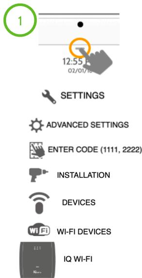
Open settings tray, touch settings, advanced settings, type valid code, touch installation, devices, WI-FI devices, IQ WI-FI
