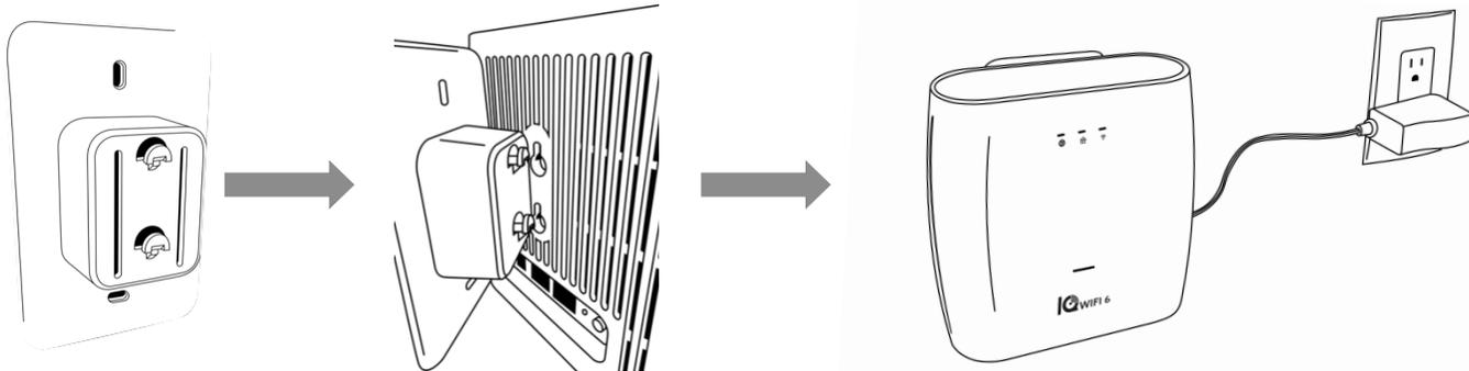
If mounting to the wall please use drywall anchor screws OR the provided sticky tape on the mounting bracket. Verify that the mount provided is oriented with the space in the tab UP.
