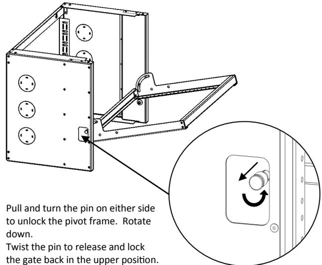
Pull and turn the pin on either side to unlock the pivot frame. Rotate down.
