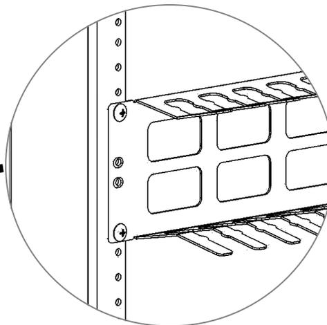
Mount forward facing or rear facing using standard rack screws (and cage nuts if necessary).
