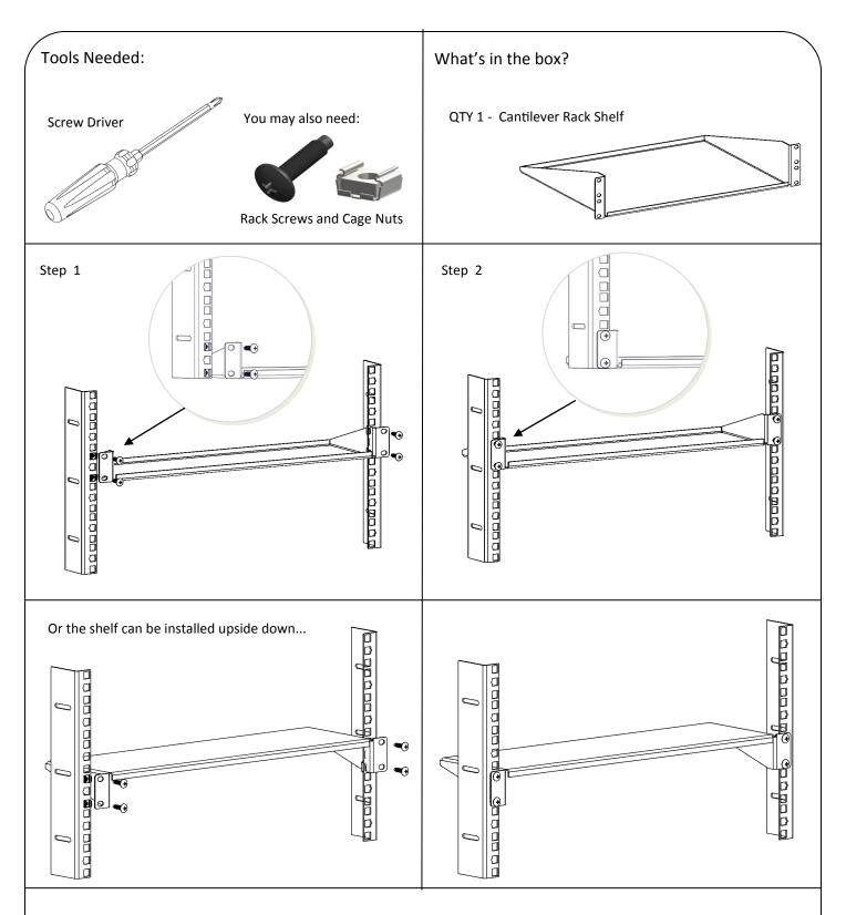
\*\*For the best results install a rack screw in every mounting hole of the rack shelf.\*\*
