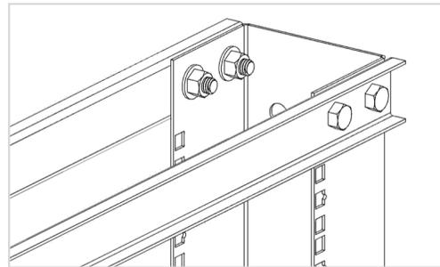
Assembly Tip: Hand tighten all bolts until the entire rack is assembled. Then go back and tighten them with the wrench.
