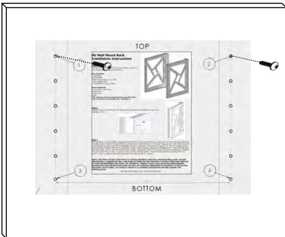
1. With a electronic stud finder, locate the exact center of a wall stud where you would like to mount the rack. Mark the wall with a pencil where the top of the wall rack will be.
