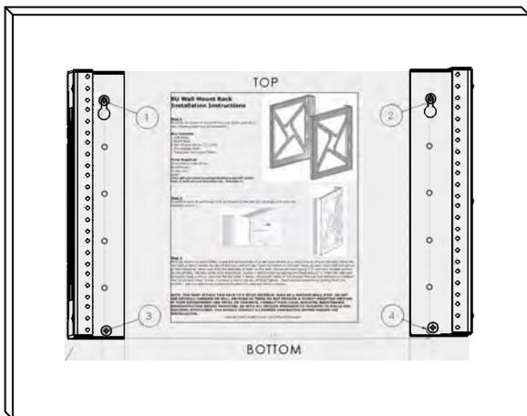
1. Leaving the template in place, hang both sides on the screws through the keyhole provided at the top of each base.
