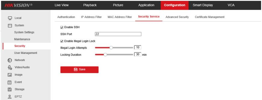
Figure 4-1 SSH Enable Interface
