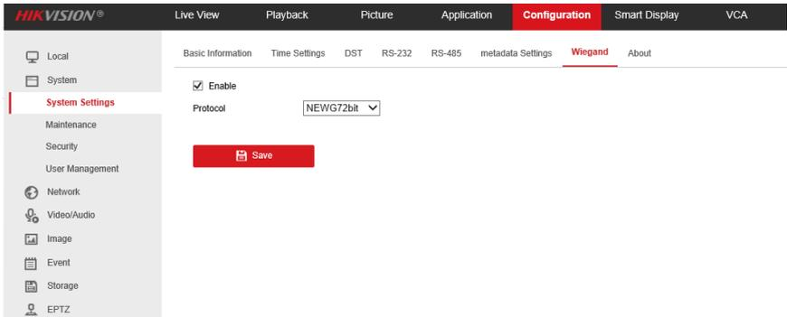
Figure 3-9 Wiegand Configuration Interface
