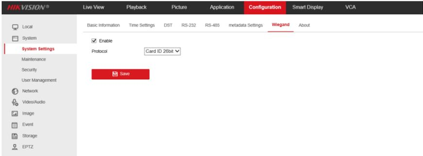
Figure 3-3 Wiegand Configuration Interface
