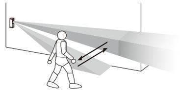
17 After walk test is complete, set DIP switch 1 (WALK TEST MODE) from "ON" to "OFF".
