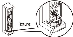
3 Hold the top of the bracket and remove the main unit.
