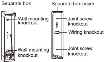
7 Pull the connectors through the wiring knockout.
