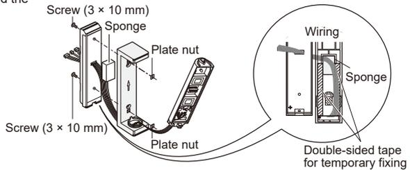
9 Hold the top part of the bracket and mount the main unit.
