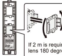
If 2 m is required, rotate the lower lens 180 degrees.
