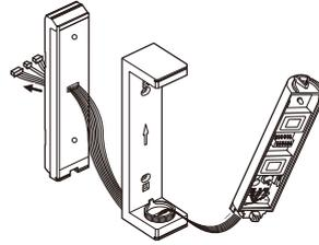
8 Attach the separate box cover and the bracket.
