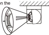
14 Determine the detection length. (2 m or 5 m)
