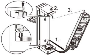
10 Mount the separate box on the wall.
