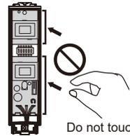
Do not touch the PCB except for the DIP switch.
