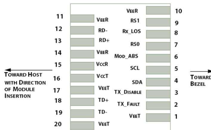
**Figure 3: Module Contact Assignment**
