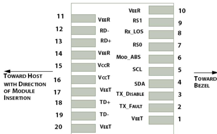
**Figure 3: Module Contact Assignment**
