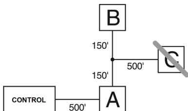
**Figure 1-1 Corbus Wiring**
