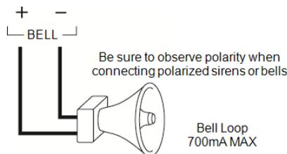
**Figure 1-5 Bell Wiring**
