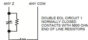
**Figure 1-4 DEOL Wiring**
