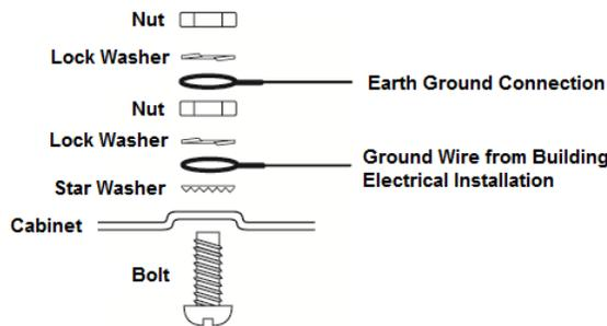
**Figure 1-7 Ground Installation**
