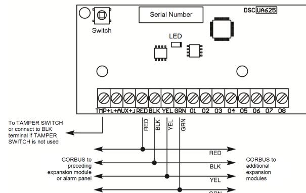
**O1 to O8 -** Wire the positive lead of the device to either AUX terminal and the negative lead to the required output terminal (O1 to O8).
