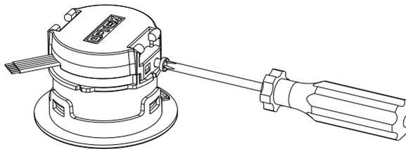
Close the base cover, and fasten the screw to fix the cover.
