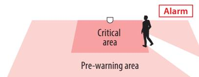
Detection area generating an alarm signal immediately and the one generating a pre-warning signal.
