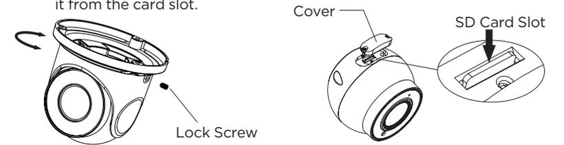
**Resetting the camera:** To reset the camera, use the tip of a paper clip or a pencil and press the reset button at the base of the camera. You will need to loosen the lock screw to disassemble the camera module from the base and access the control panel. Pressing the button for five (5) seconds will initiate a camera-wide reset of all the settings, including network settings.
