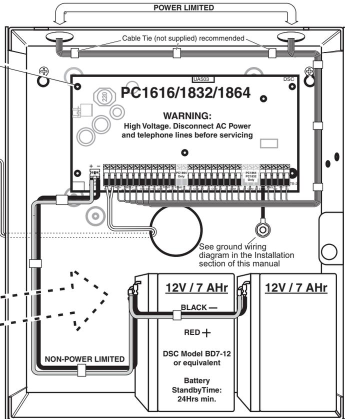
**WARNING:** Incorrect connections may result in PTC failure or improper operation. Inspect wiring and ensure connections are correct before applying power.
