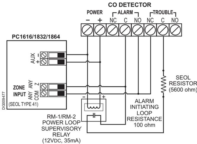
The following hardwired CO Detector models can be used with PC1616/PC1832/PC1864 v4.5 (and higher) control panels:
