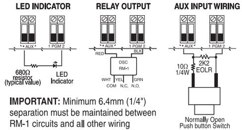
**IMPORTANT:** Minimum 6.4mm (1/4") separation must be maintained between RM-1 circuits and all other wiring
