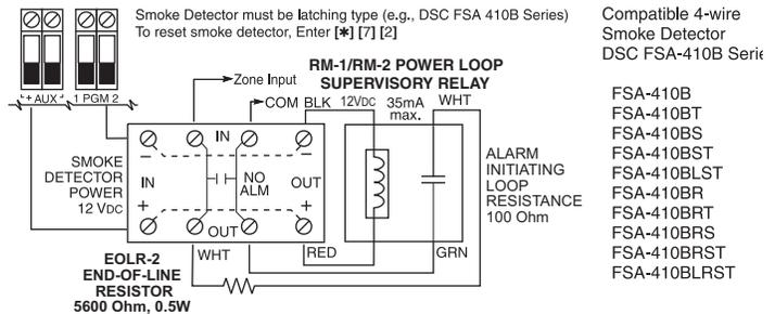
Compatible 4-wire Smoke Detector DSC FSA-410B Series
