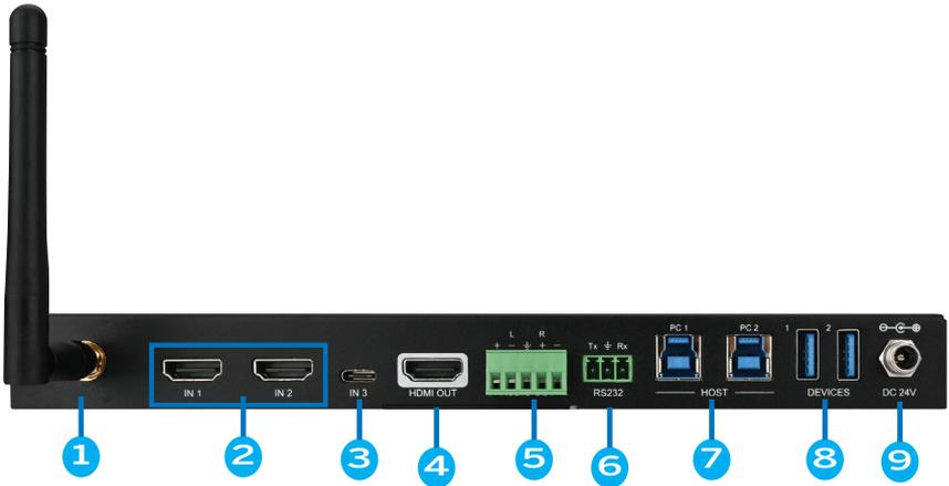
1. External Antenna: Connect to the provided external antenna for Miracast/Airplay Wireless Input connectivity
