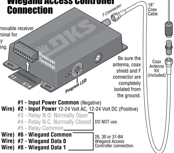
Be sure the antenna, coax shield and F connector are completely isolated from the ground.
