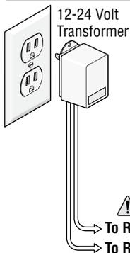
**Separate Power Source:** Connect 12 - 24 Volt AC or DC power to terminals #1 and #2. Use minimum 18 AWG wire to power the receiver.
