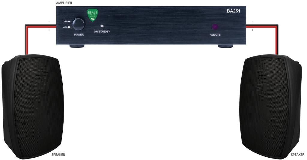
The speaker terminals on the speaker are red on one side and black on the other. Connect to the red terminal of the amplifier to the speaker (+), and connect the black terminal of the amplifier to the speaker (-). Connect each speaker to make sure there is not inverted polarity (+ goes to -). If the polarity of the speakers is reversed, the sound will be unnatural and will play without bass.
