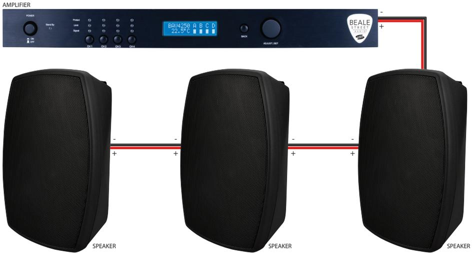
The total number of speakers multiplied by the tap value cannot exceed the output power (in watts) of the 70V/100V amplifier. The example below shows 3 total speakers. Using the 10W taps, you will need an amplifier with at least 30W (3 speakers x 10W tap).
