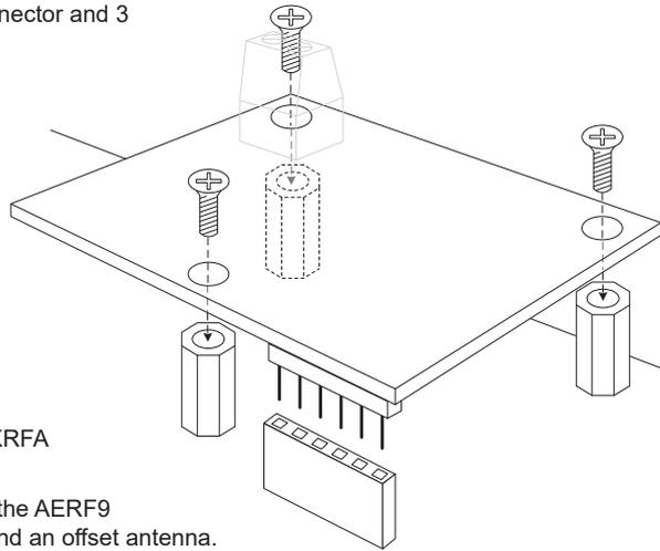
4. Two antennas are included with the AERF9 transceiver; a straight antenna and an offset antenna. The straight is to be used when the transceiver is installed on the E27 board. The offset antenna is to be used when the transceiver is installed on the AEXRFA adapter. Install the appropriate antenna in the ANT screw terminal located in the upper left corner of the AERF9 wireless transceiver.
