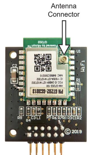
3. Locate the antenna connector on the AEWF adapter (see image to the right). Plug the antenna cable onto the antenna connector. To avoid damage, care should be taken to limit excessive removal and reconnection of the antenna cable.
