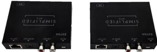
The EXTDA is a 100m (at 192kHz./24-bit resolution) audio over category cable extender. Optical (S/PDIF) and RCA analog formats are supported either singularly or both at the same time. The RX or TX portion powers both devices. The RX can select RCA or Optical input from the TX for the RCA output portion. If using optical, the display's audio settings need to be set to PCM. Greater distance (up to 300m) can be achieved with lower audio resolution settings.
