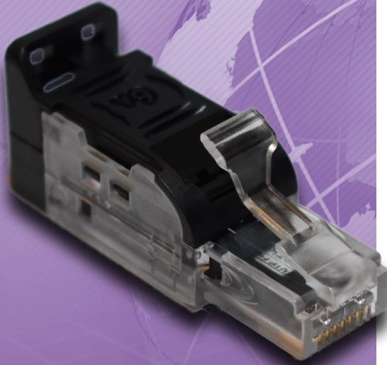
The **106260 CAT6A-rated PoE++** connector features a simple 2-piece design and only requires basic wiring tools to terminate in the field. Compatible with cables ranging from 6.0mm to 8.5mm and conductor sizes of 26 AWG to 23 AWG. This connector is compliant with CAT6A/CAT6/CAT5e requirements as well as the PoE++ type 4 standard up to 90W.
