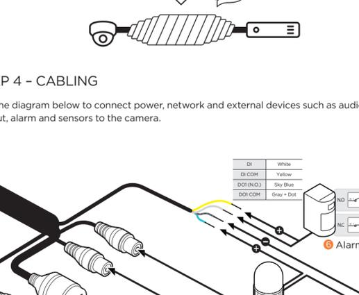
**NOTE:** Cables with ø4.5mm to ø5.5mm thickness should use the black rubber ring. Cables over ø5.5mm in thickness should use the white rubber ring.
