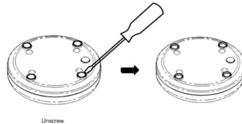
2. Remove the screws from the case to access the battery cell.
