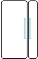
The **PWD** Window/Door Transmitter is a magnetic sensor device designed to fit seamlessly alongside a door frame or windowsill. When the door or window is opened, the magnetic contact is disrupted and the sensor transmits a notification to the panel.
