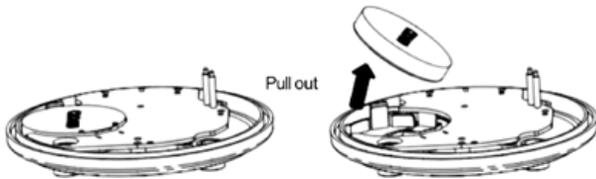
Replace with one **CR2450** (3.0V, 600mAh) cell.
