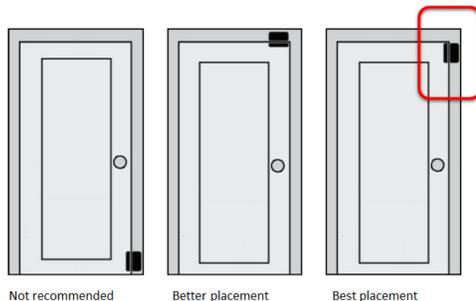
The transmitter and magnet each have a slightly engraved line to denote their best alignment to function properly. If a "closed" transmitter and magnet are misaligned, the sensor will not report correctly. See illustration at right that displays the correct alignment.
