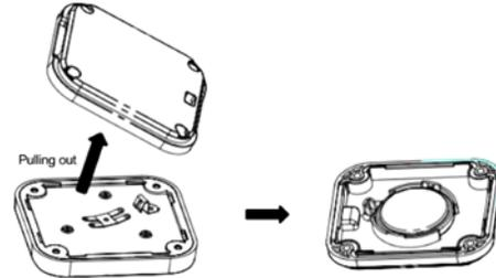
4. Remove the old cell battery and insert a new cell, observing polarity.
