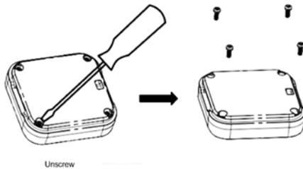
3. Remove the rear cover, then remove the cell battery.
