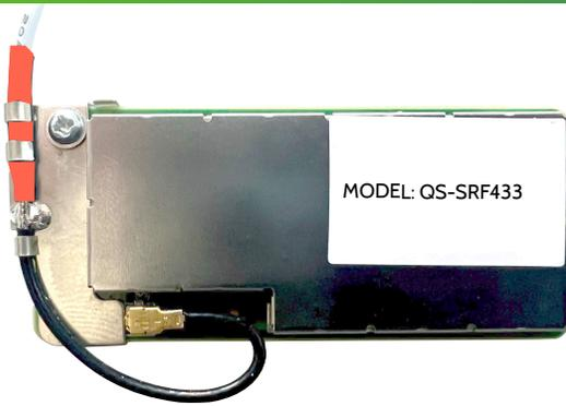
The IQ Card-433 can be installed in to “Slot 3” of your IQ Panel 4, IQ4 Hub or IQ4 NS to enable support of approved legacy 433 MHz SRF sensors.
