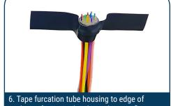
5. Tape furcation tube housing to edge of the surface so tubes hang down to floor. Untangle fibers so each can be separated back to the point where it exits the housing assembly.
