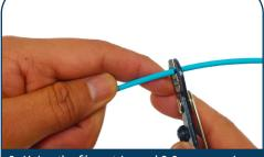
3. Using the fiber strippers' 2.0 mm opening, remove the jacket at marking so that the exposed fiber is equal to the breakout tubing and assembly plus 6" or 15 cm.
