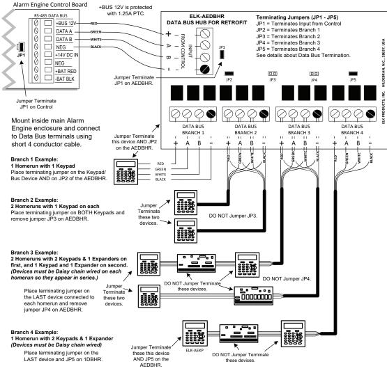
The above examples are intended to show the flexibility provided by the 4 data bus branches of an AEDBHR. The number and types of devices used on each branch is up to the Installer.
