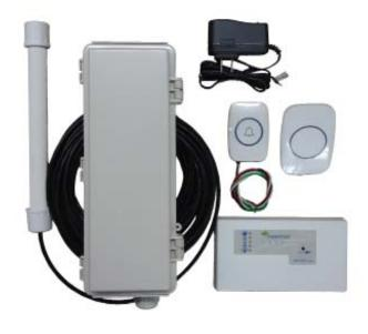
The LP2C is a complete vehicle detection system. It utilizes the LP2 2-zone processor which allows for multiple possible configurations. With one sensing probe you can cover one driveway in non-directional mode. With two sensing probes you can cover two driveways in non-directional mode or one driveway in directional mode. By adding a second transmitter when using two probes you can have an individual output per driveway or per direction.
