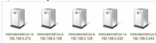
Once the PC discovered the NVR, double click on the icon to open the NVR’s web client. Enter your User ID and Password to login and click ‘Connect’ to connect.
