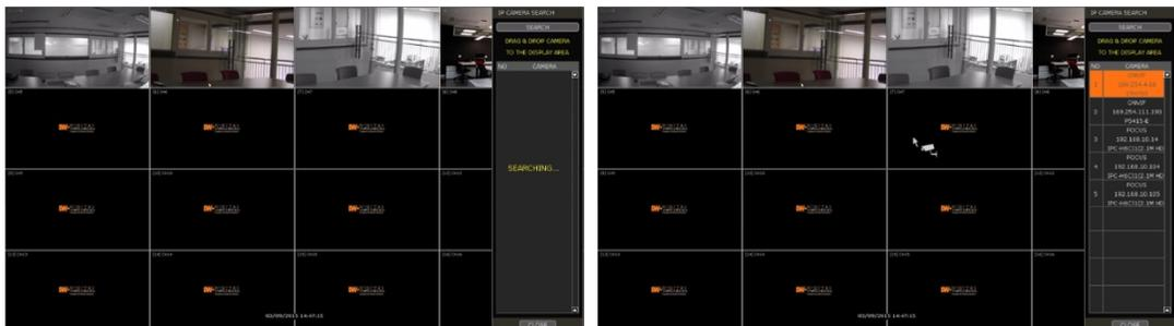
2. Select a camera and while clicking on the camera, drag it to a channel to assign it.
