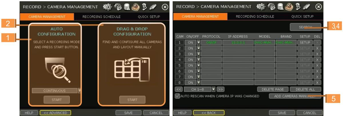
The NVR supports three ways to search and register cameras to the NVR. The AUTO CONFIGURATION option allows the NVR to scan the network and automatically register the first cameras it finds to the available channels.
