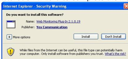
3. To avoid download restrictions for the Active X file, make sure that Active X controls are enabled in the web browser's security settings. Go to "Tools > Internet Options > Security > Internet > Custom Level" and enable all Active-X controls and plug-in.
