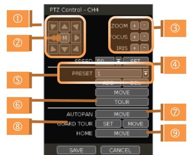
TOUR: Set the camera to move between preset positions in order. The camera will keep running the tour until it manually is disabled.
