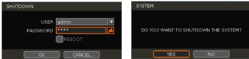
**Note** Users can input passwords by the virtual keyboard, IR remote control, or front numeric buttons (if available).
