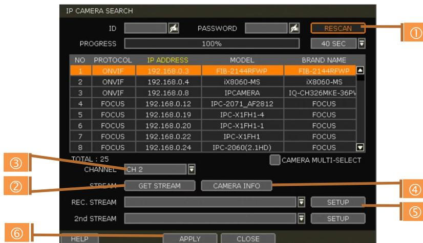
3. When [GET STREAM] is selected, the NVR will assign a channel number to the selected camera. Users can also select a specific channel number from the drop-down options.
