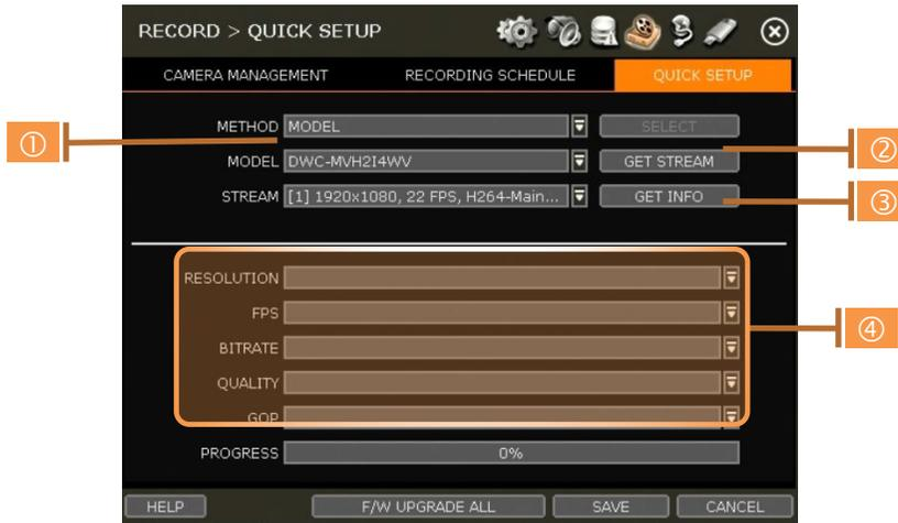
1. Select the method and model to setup. All cameras with the same model name will be selected.
