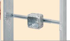
Mount SliderBar on studs with #8 x 1/2" screws. Position box on bar. Tighten screws inside box.
