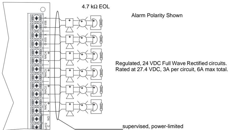
Figure 4.44 Class B Notification Appliance Circuit Wiring
