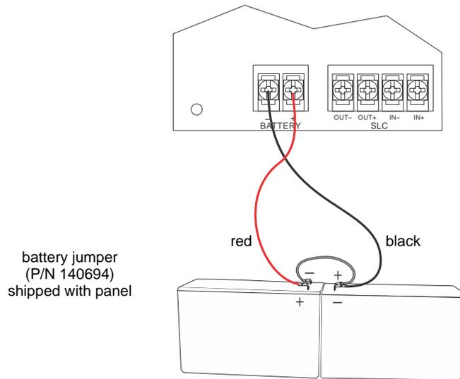
Figure 4.6 Battery Connection
