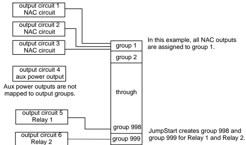
Figure 7.3 Assigning Output Circuits to Groups (Example)
