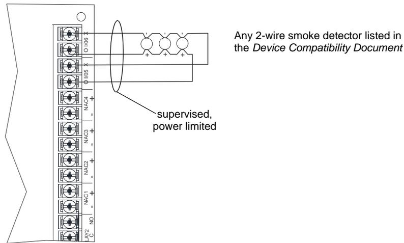
Figure 4.49 Two-Wire Class A Smoke Detector Connections
