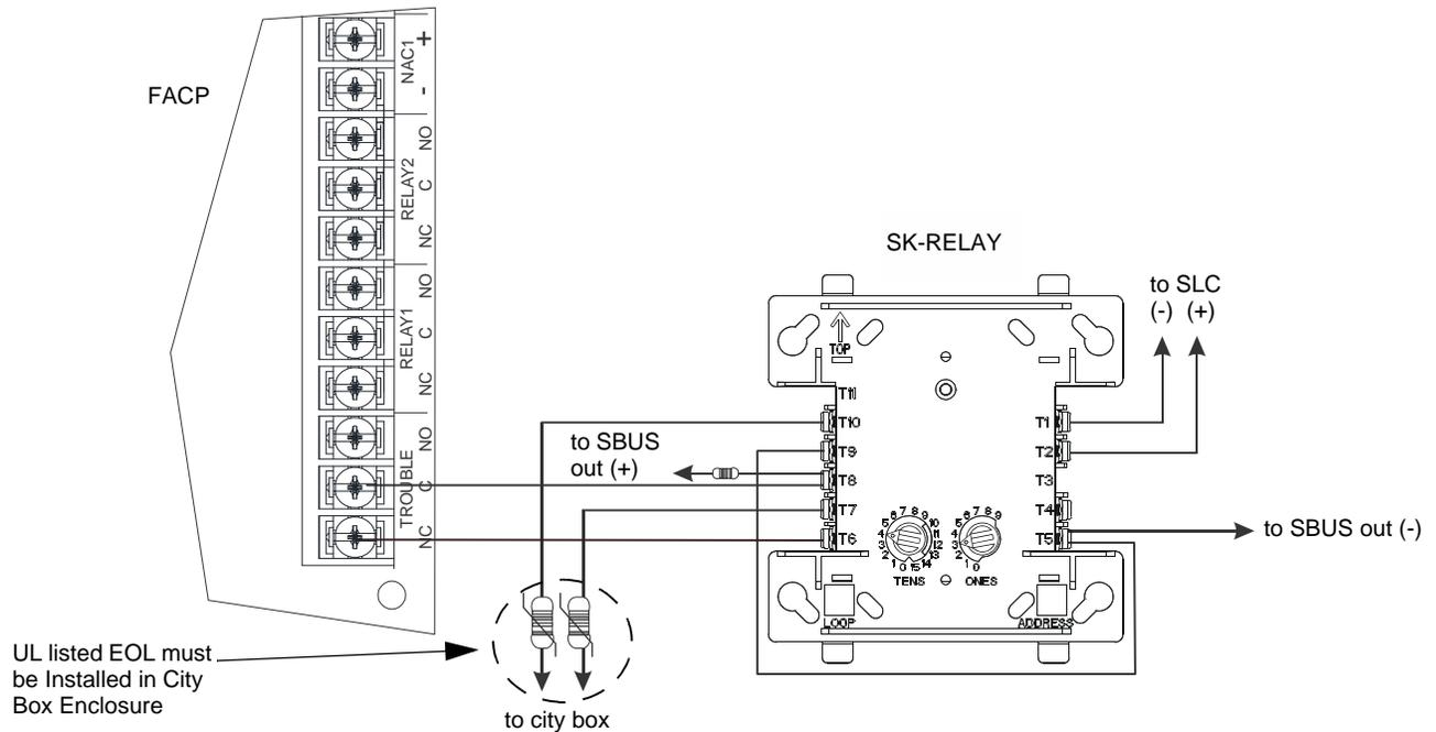
Figure 4.56 Relay Module for City Box Connection
