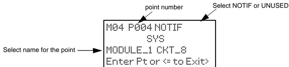
**Figure 8.6 Programming Points Screen for the EVS Amplifiers**
