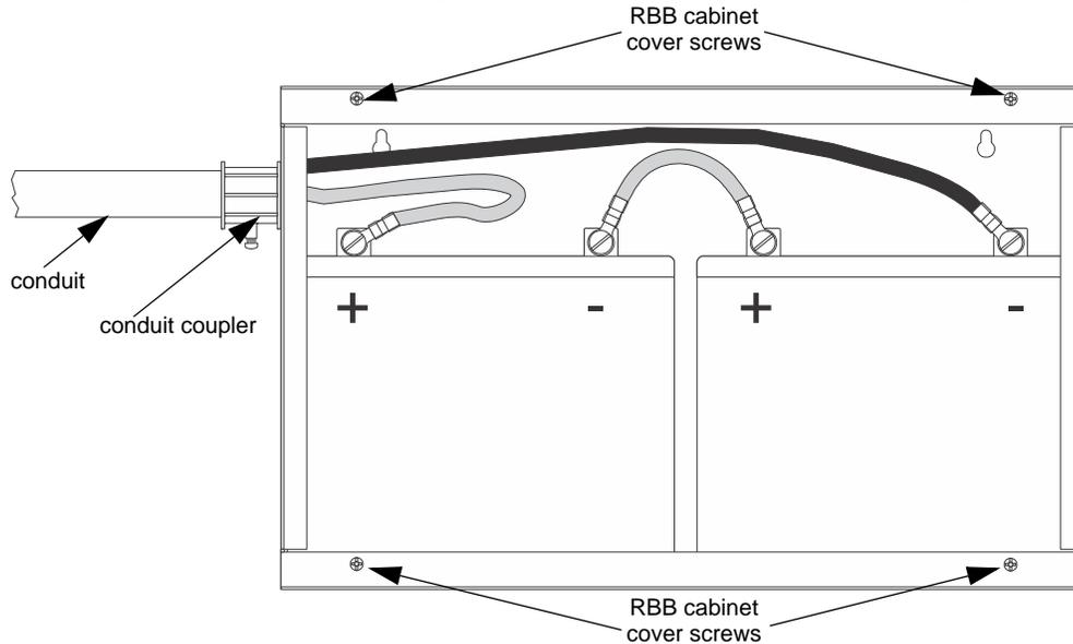
**Figure 4.9 Battery Connections in the RBB Cabinet**
