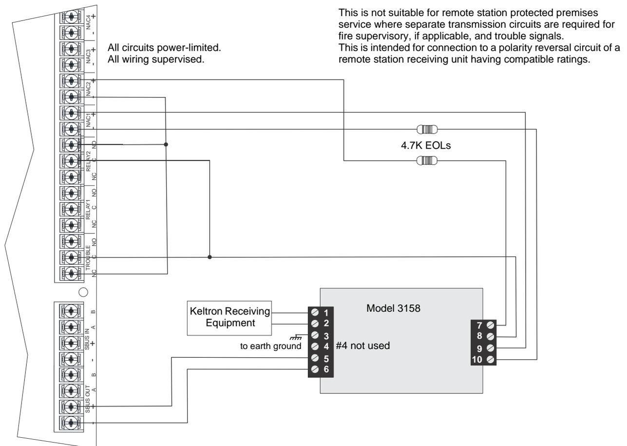
Figure 4.54 Keltron 3158 Connection to Control Panel
