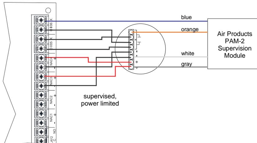
Figure 4.51 Class A 4-Wire Smoke Detector Connections
