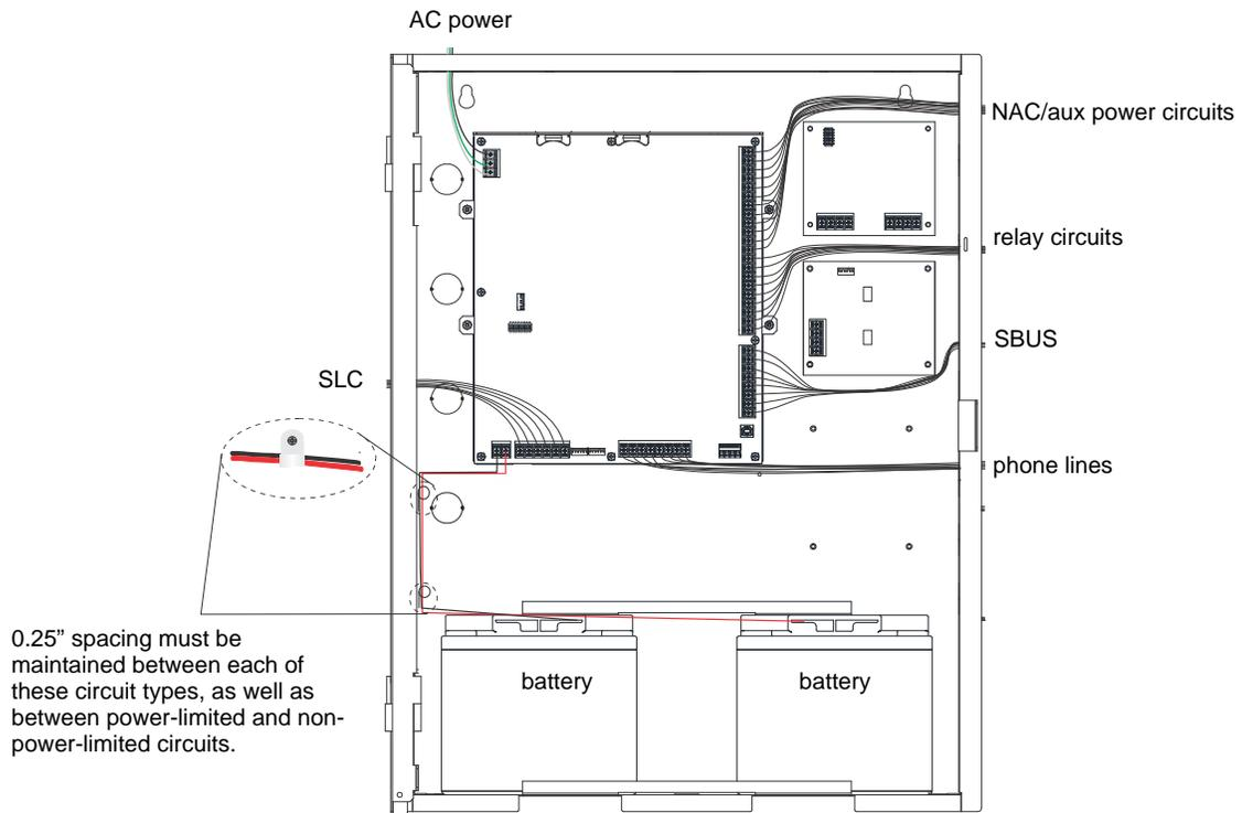
Figure 4.4 Wire Routing Example for 6820EVS
