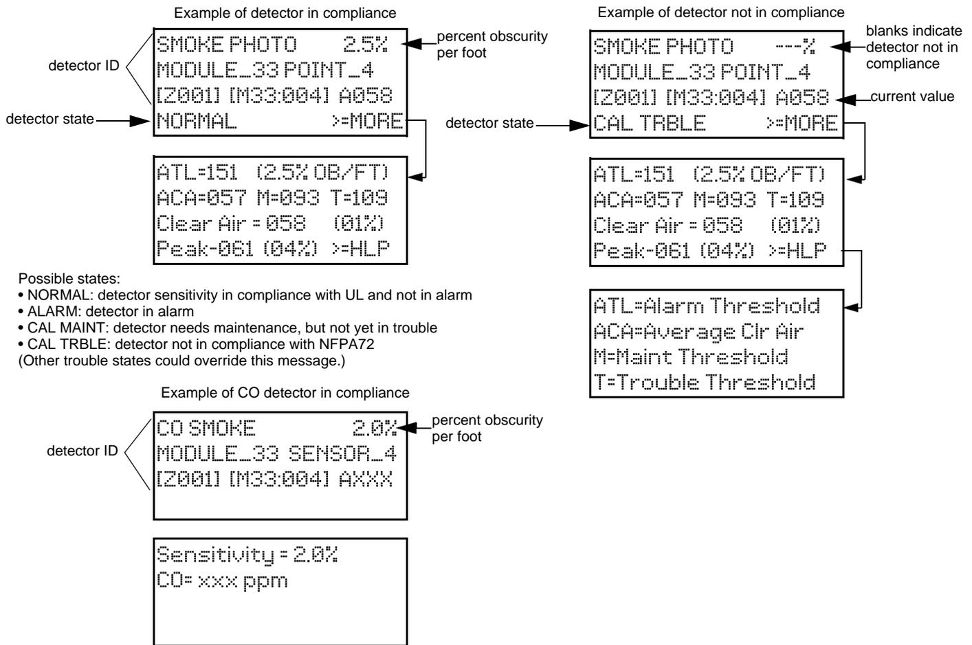
Figure 9.5 Checking Detector Sensitivity Compliance on 6820
