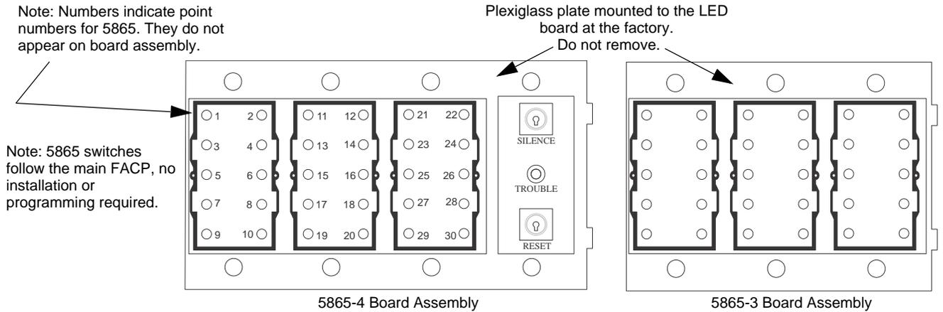
**Figure 4.38 5865-3 and 5865-4 Assembly (Front View)**
