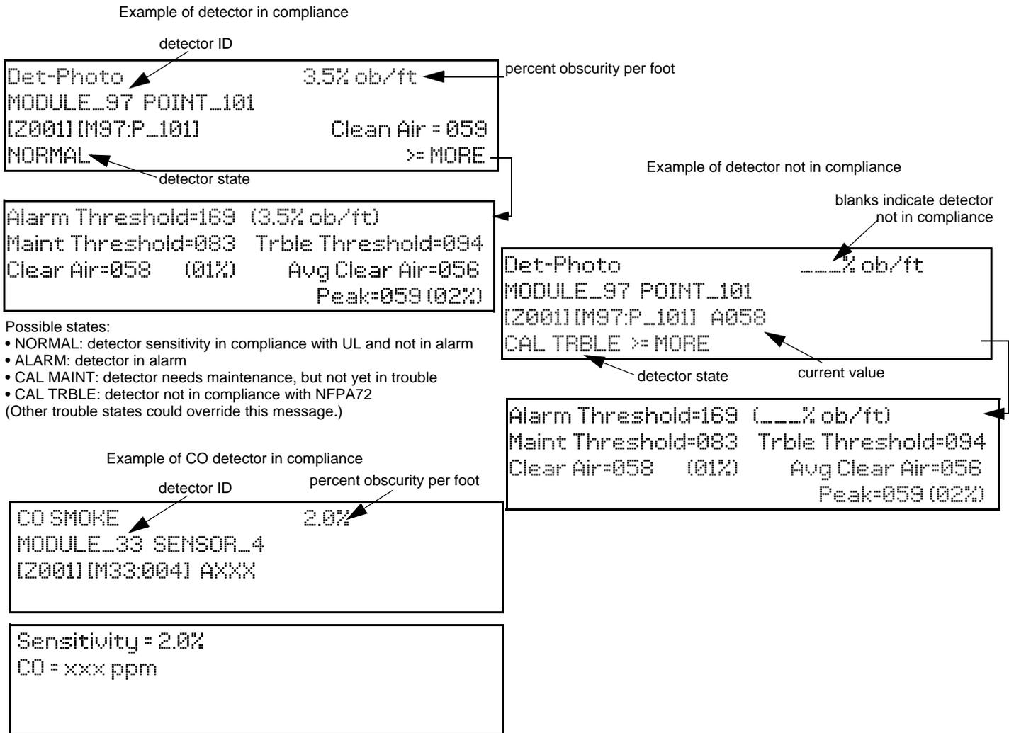
**Figure 9.6 Checking Detector Sensitivity Compliance on 6820EVS**
