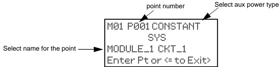
**Figure 8.5 Programming Points Screen for the 5496 Module**
