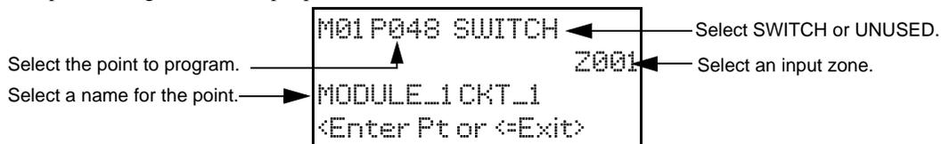
**Figure 8.4 Programming Input Points Screen for 5880 and 5865 Modules**
