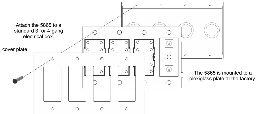
Figure 4.40 5865 Mounting Example
