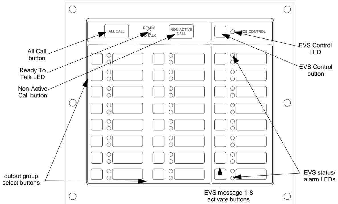
Figure 10.1 Front View of EVS Keypad
