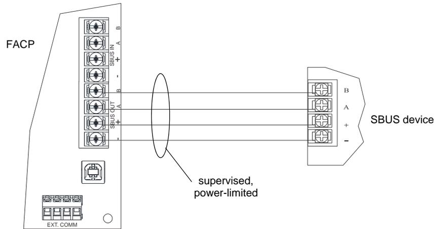
Figure 4.12 SBUS Class B Wiring
