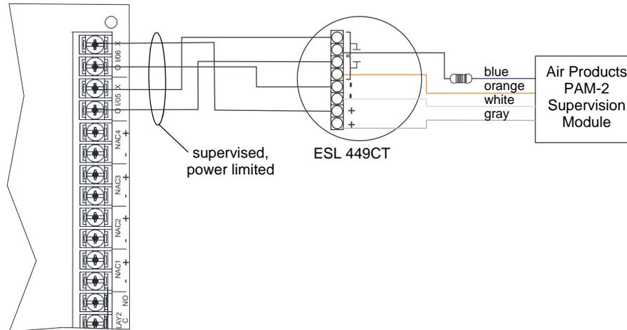
Figure 4.50 Class B 4-Wire Smoke Detector Connections
