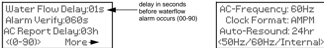
**Figure 8.11 Water Flow Delay Programming Screen**
