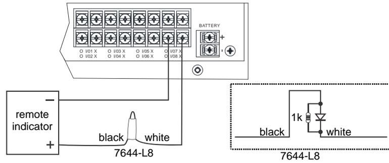
**Figure 4.58 Polarity Reversal Connection Using the 7644-L8**
