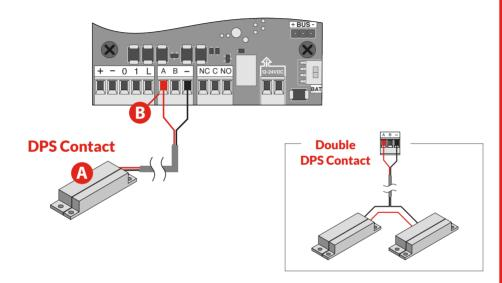
A DPS (Door Position Sensor) - The DPS is mounted on the door frame with a 22/2 wire running from the DPS to the controller. Wire the DPS to the controller as shown above. For reporting double doors, wire the two-door position in series and connect to the controller.
