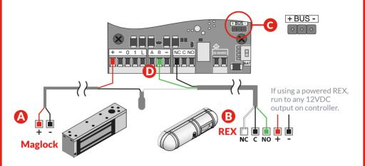
A Maglock - When installing a Maglock, it is typical to install a REX (request to exit) at the door for free egress. Run an 18/2 wire from the maglock to the controller and REX as shown.
