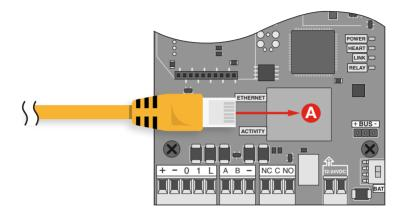
Ethernet - All Red controllers come with a built-in RJ45 connection for network connectivity. Once connected, the Red controller is
