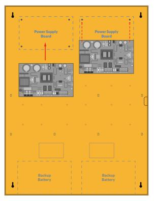
**Mount** - Line up the power supplies with the top mounting brackets in the enclosure. Using the supplied screws, fasten the power supplies to the enclosure.
