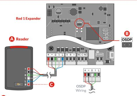
A **Reader -** The reader is mounted at the door with a 22/5 or 22/6 wire running to the door controller. Wire the reader to the controller as shown above. Be sure to check the polarity and voltage prior to powering the controller.
