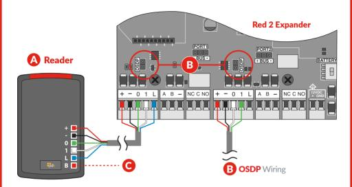
A Reader - The reader is mounted at the door with a 22/5 or 22/6 wire running to the door controller. Wire the reader to the controller as shown above. Be sure to check polarity and voltage prior to powering the controller.
