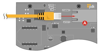
Ethernet - All Red controllers come with a built-in RJ45 connection for network connectivity. Once connected, the Red controller is Self-Discoverable from pdk.io using IPV6. Alternatively, you may use IPV4 or assign a static IP using pdk.io if desired.
