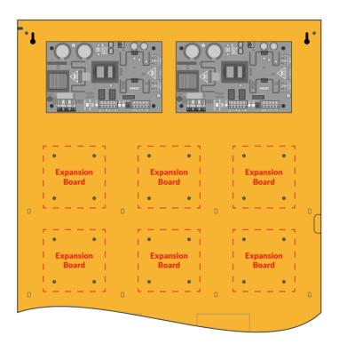
**Mount -** Select your desired mounting location within the enclosure. Line up the expander board with the desired mounting brackets. Using the supplied screws, fasten the expander board to the enclosure.
