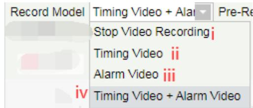
⑤ Select Pre-Record Time: When the record model is in **Stop Video Recording** or in **Timing Video**, the pre-record time should be **"No Pre-Record"** by default.
