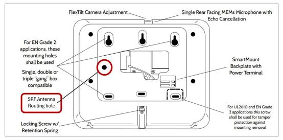
**Wall mount:** Use the backplate as a template to mark the appropriate locations for the mounting screws and the legacy SRF antenna. Drill a 1/4" (or larger) hole in the wall for the legacy SRF antenna. Feed the external legacy SRF antenna into the wall when mounting the panel to the backplate.
