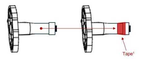
The PG9WLSHW8 / PG9HRDW8 hardwired to PowerG wireless module has a front and rear tamper. The front tamper boot can be accidently knocked off if the cover is not handled with care.
