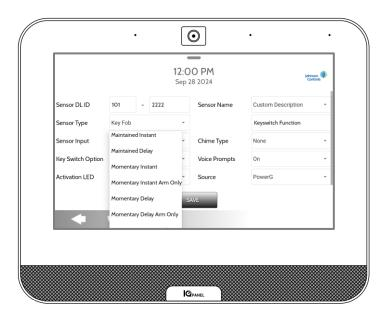
The IQ4 v4.5.0 and higher panels have a feature that can be used to arm and disarm the system through a "keyswitch" operation. This is often used to arm or disarm the system from a trigger from a 3<sup>rd</sup> party application, such as a card access system, home automation system or an old fashion keyswitch.
