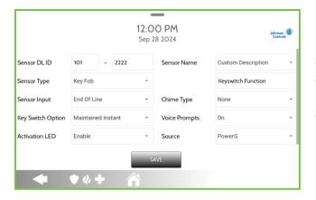
Sensor Type = 'Key Fob' Sensor Input = (as needed) Key Switch Operation = (as needed) Sensor Name = (as needed)
